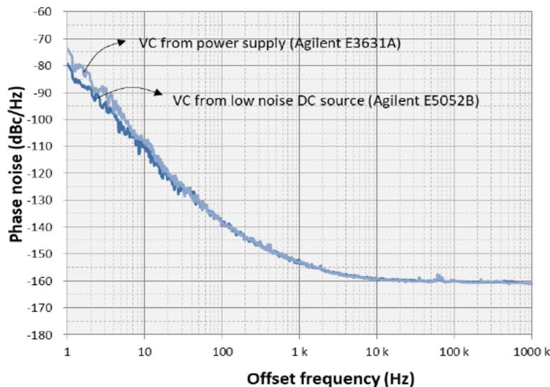
**Figure 10 Comparison of phase noise measurement using different DC source from the signal spectrum analyzer (Agilent E5052B) and the power supply (Agilent E3631A)**
