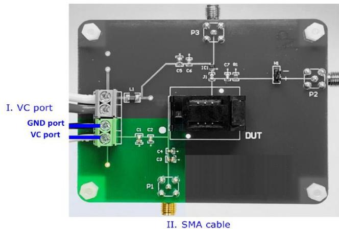
**Figure 4 – VC connection by [I] VC port and [II] SMA connector**
