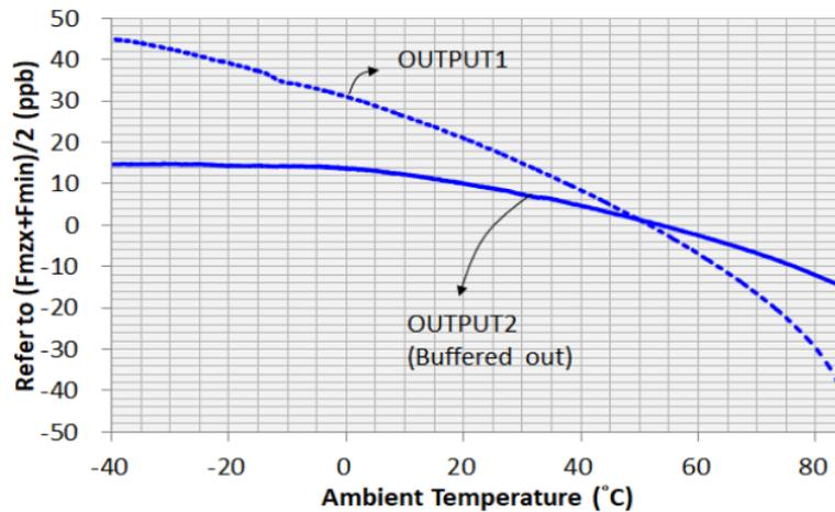
Figure 7 – Temperature stability comparison between buffered output (OUTPUT2)
