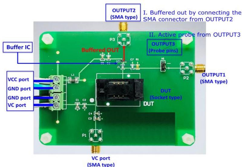
Figure 8 – Output connections by [I] directly using buffered out from OUTPUT2 (P3)
