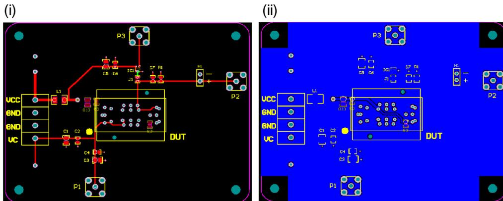
Figure 3 – The layout of OCXO EVB (i) top & (ii) bottom layer
