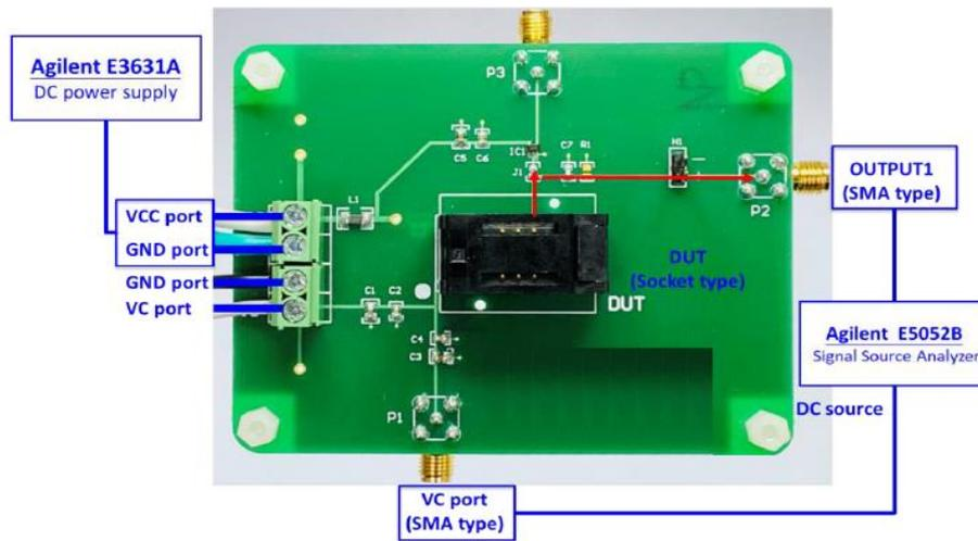
**Figure 9 – Connections of phase noise measurement by using DC source from Agilent E5052B.**
