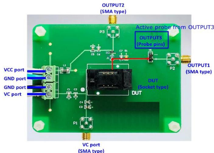
Figure 6 – Frequency and waverform measurement
