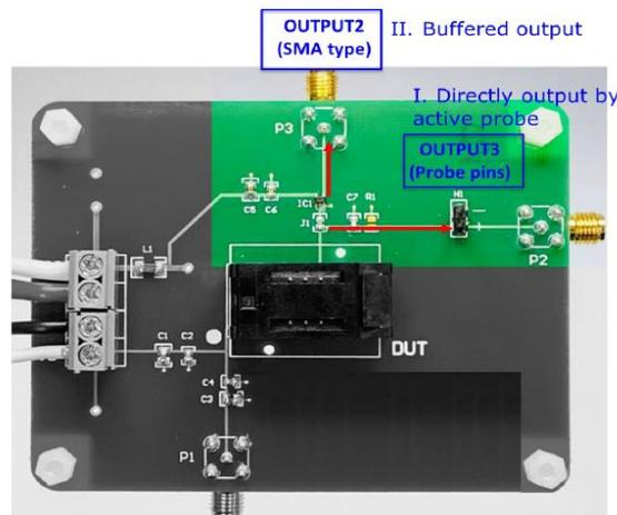
**Figure 5 – Output connections by [I] active probe and [II] buffered output by SMA**
