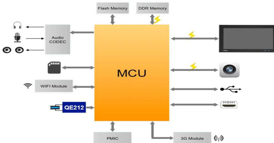
The block diagram above shows a very typical application (Tablet PC), which supports numerous interfaces. The EMI / RFI compliance while also staying in compliance with the USB 2.0 specification is addressed by the usage of a QST Active EMI reduction IC (QE212) at the clock source of the ASIC (MCU). This IC is subsequently replaced by a 1st-Gen Active EMI reduction IC from a competitor, configured to achieve comparable EMI / RFI benefits and the comparative results of
